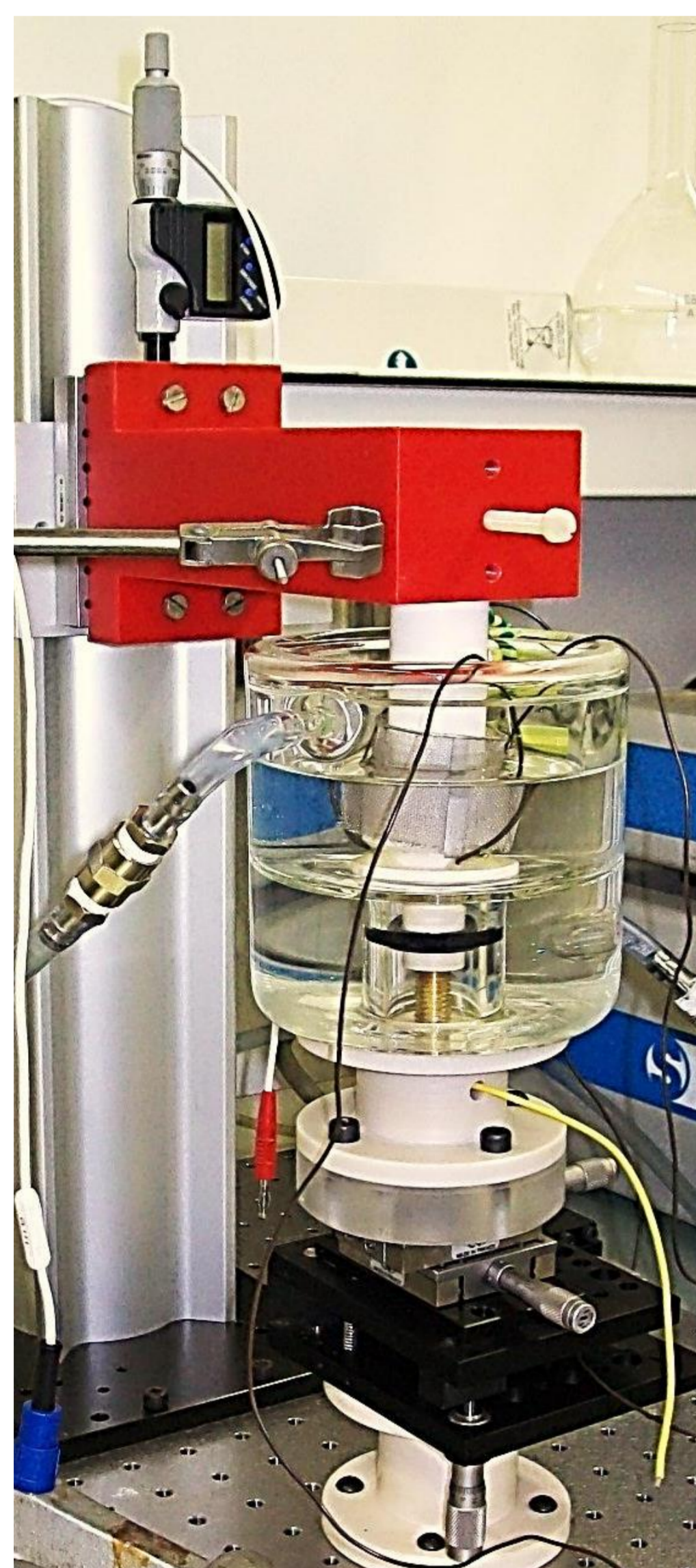
Thin layer cell and electrodes, used to reproduce crevice corrosion conditions
