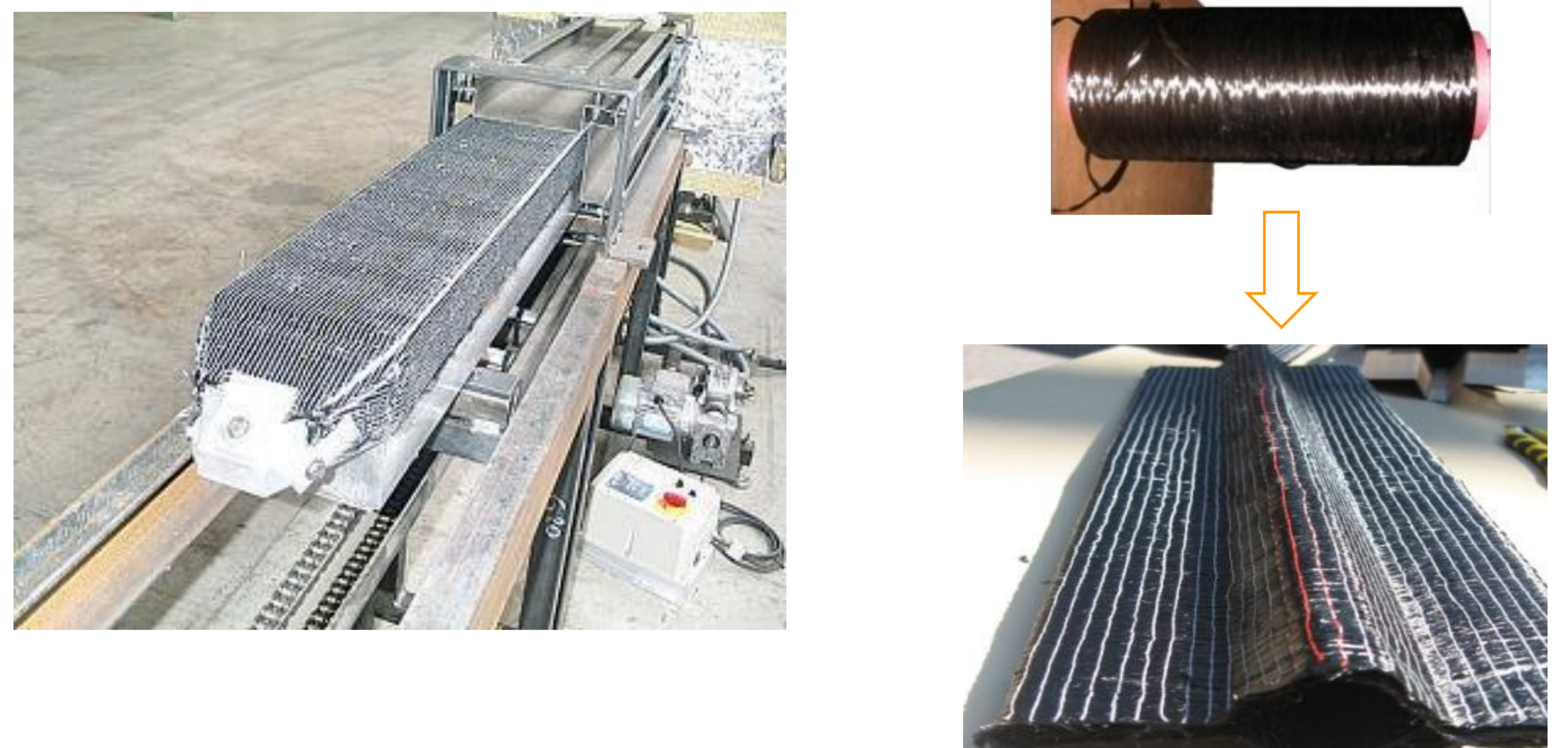
Preforming of a beam and a stiffener
