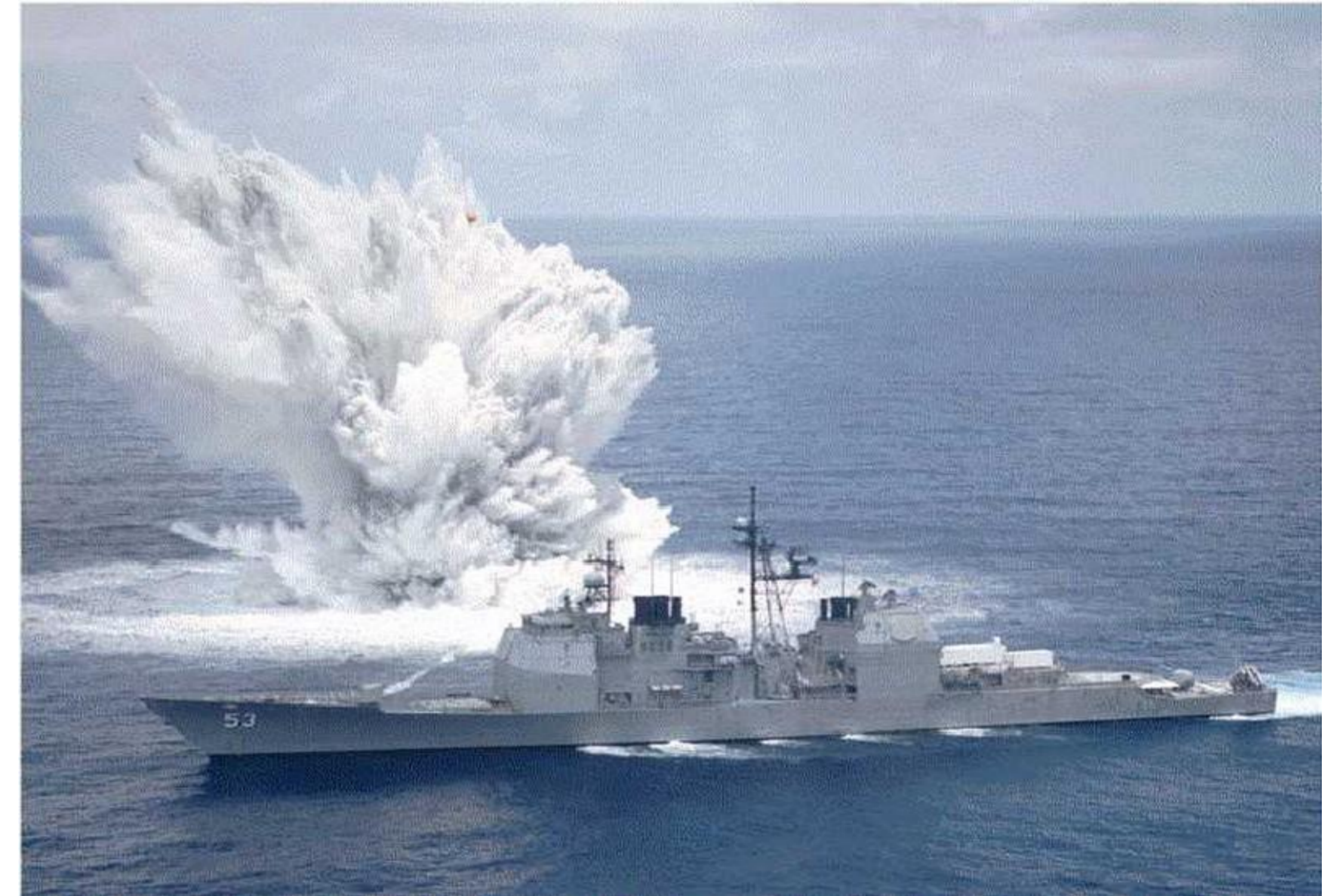
Ship submitted to underwater explosion
